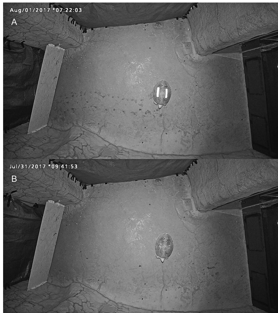
Figure 1. Photos from the Panasonic surveillance camera taken during experiments with a female northern river terrapin ( Batagur baska ). The carapace size of the terrapin is 48 \times 36 cm. Pictures were taken from a height of 5 m. (A) With reflective tape ( 5 \times 20 cm); (B) without tape.
